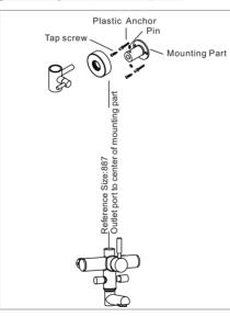
Install the mounting part as above picture shown, making sure that the center point of mounting part isperpendiculartooutlet port of mixer body
