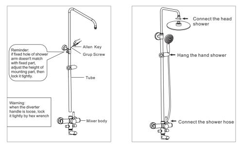
Insert the tube with the cap and mounting part, connect the tube and mixer body by rotation method to make sure tube to be parallel with wall, then lock it tightly by  $\varphi$  2.5 allen key.
